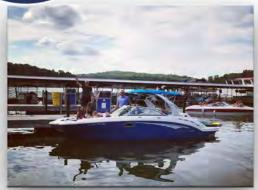
INBOARD / OUTBOARD (I/O) - The engine unit is located inside the boat and has a sternmounted prop unit; it allows for a longer swim platform on the stern, which resides over the prop.
